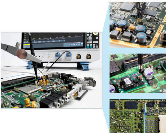
2 GHz coax solder in pigtail is shown connected to channel 2, while a passive 350 MHz browser with bypass cap clip and ground spring is shown to the right
