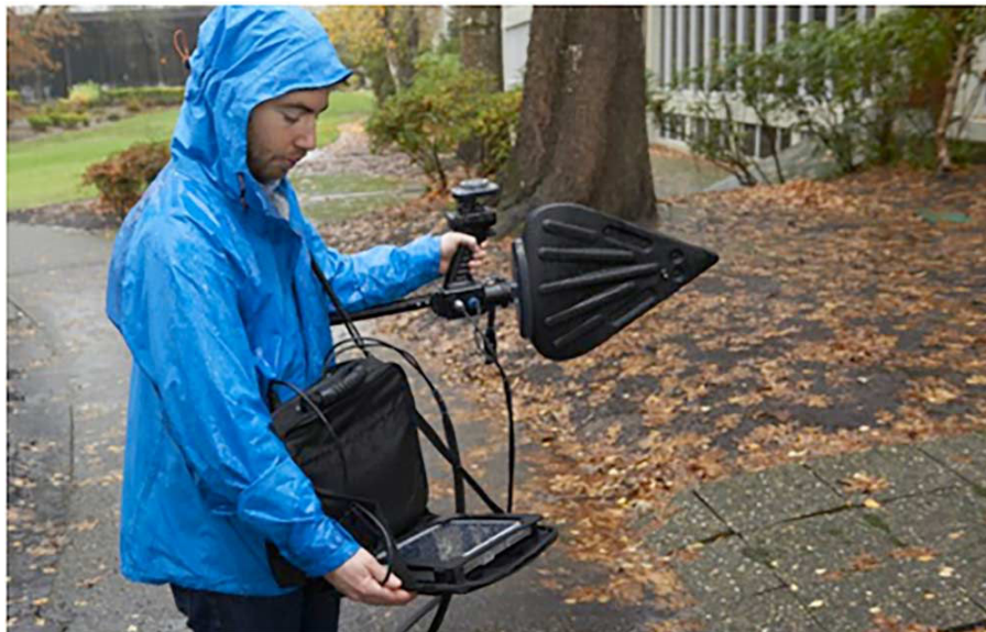
Figure 9. The Tektronix spectrum analyzer with mapping/triangulation and Alaris DR-A0047 antenna. Photo, courtesy Tektronix.
