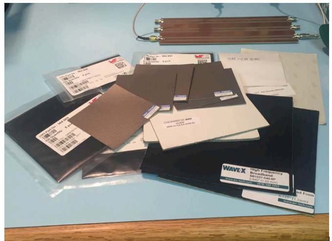
Figure 1: My collection included a variety of ferrite absorber sheets from different manufacturers
