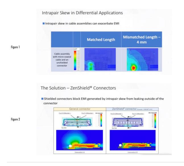
connectors. We compared matched lengths, a slight mismatch of one millimeter, and a larger mismatch of four millimeters.
