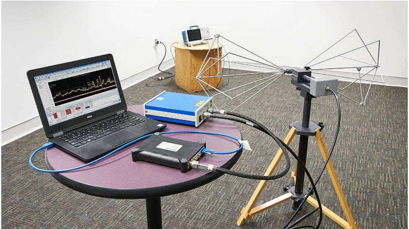
Figure 3: Typical radiated emissions pre-compliance test setup in a large room. The spacing between the EMI antenna and equipment under test is 3 m.
