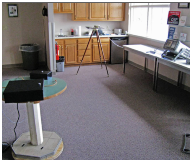
Figure 3: An example of a 3m pre-compliance test set up in a large conference room. Note the DIY turntable for helping maximize emissions.
