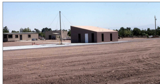
Figure 2 - A typical open area test site (OATS).
