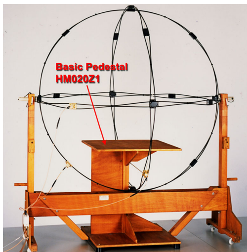
R&S®HM020 with a loop diameter of 2 m. Such LLAS can be used for EUT with a largest dimension of up to 1.6 m.
