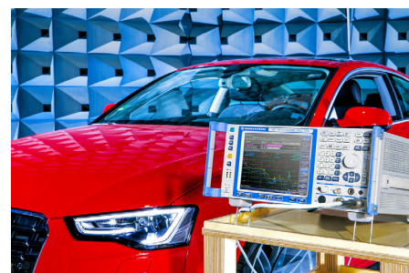
CISPR 25 covers interference caused by the vehicle to equipment mounted within the vehicle, such as a radio or GPS receiver.
