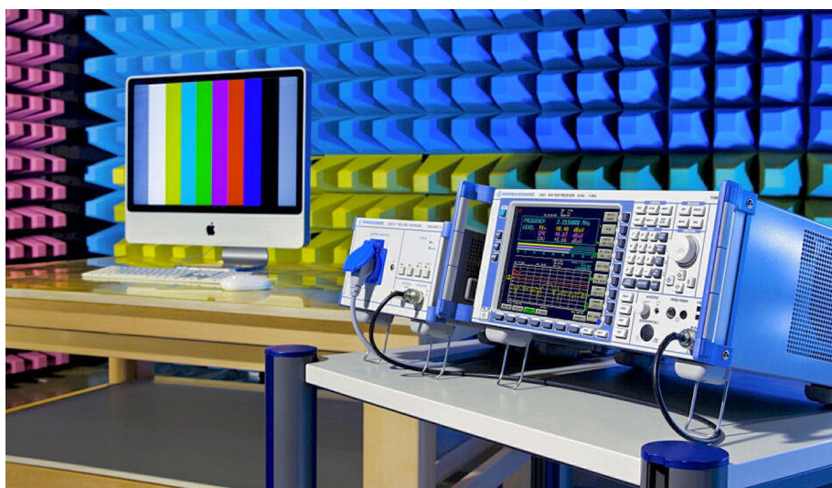
Conducted EMI test in accordance with CISPR 32 for a computer monitor.
