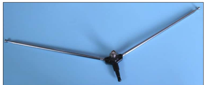
Figure 15 – Simple rabbit ears TV antennas may be used to pick up radiated emissions from a product under test. It will tune from 85 to about 220 MHz depending on how long the elements are extended. Epoxy a BNC connector to the housing and connect each terminal to the telescoping elements.
