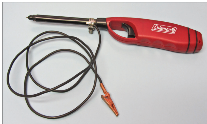
Figure 7 - The Coleman brand lighter is unique that the butane has a separate control switch with no need to empty the reservoir. Cut the metal shroud back with a Dremel tool to expose the tip and connect a length of grounding wire. It produces about 4 to 6 kV from the piezoelectric element when the trigger is pulled.
