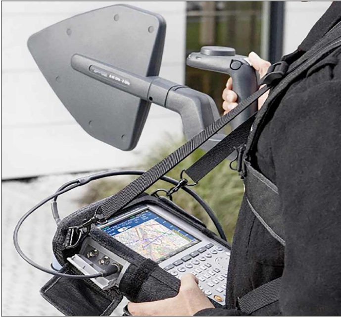
Figure 7: The Rohde & Schwarz R&S®PR100 custom spectrum analyzer with mapping and triangulation and R&S®HE300 antenna. The R&S® FSH analyzer may also be used. Photo courtesy, Rohde & Schwarz.
