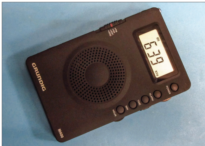
Figure 8 - An AM broadcast band radio tuned off-station is useful for detecting the "clicks" of ESD events.
