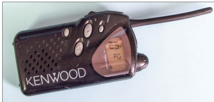
Figure 4. A typical 0.5W 465 MHz Family Radio Service two-way radio. Some other countries have similar license-free radios that may be used for simple radiated immunity testing.
