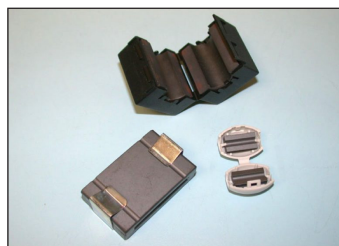
Figure 20 - Examples of various clamp-on ferrite chokes.
