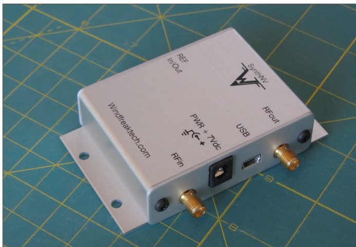
Figure 5 - The Windfreak Technologies RF synthesizer is small and can produce up to +19 dBm from 34 MHz to 4.4 GHz. It can also modulate the RF with AM or pulse.
