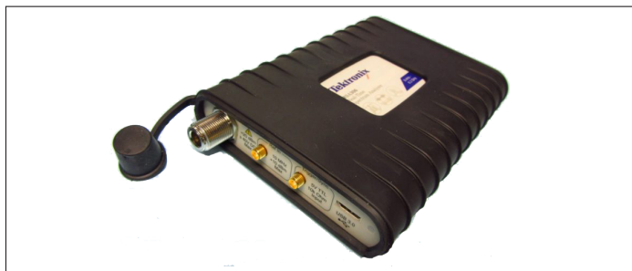
Figure 7 - The Tektronix RSA306 USB-controlled real-time spectrum analyzer covers 9 kHz to 6.2 GHz and has a real-time bandwidth of 40 MHz. The base cost is $3,489 and there are several digital modulation display options.
