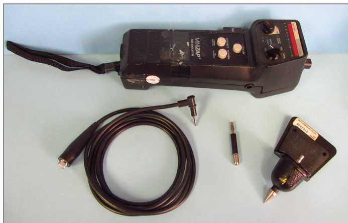
Figure 6 - The Keytek Mini-Zap is a handy handheld ESD simulator that can test up to 15 kV. The contact discharge tip is shown.
