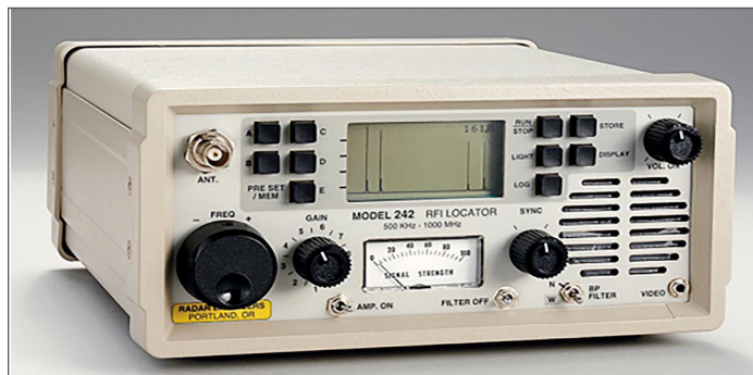
Figure 2: A signature analyzer from Radar Engineers that tunes from 500 kHz to 1 GHz and which displays an electronic “signature” of a specific interference source. Receivers such as this are used by professional investigators to track down power line noise (photo courtesy, Radar Engineers).
