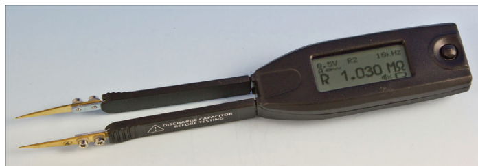
Figure 10 - The SmartTweezer RLC meter is helpful for measuring surface-mount components. Pictured is the Advance Devices model ST5, that costs $387 through their web site ( http://www.advancedevices.com ).
