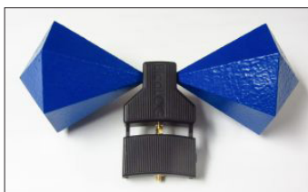
Figure 18 - A small broadband active antenna from Aaronia that is very useful for bench top troubleshooting of radiated emissions.
