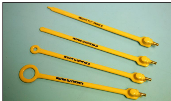
Figure 12 - A typical near-field probe set. In this picture, there are three H-field loop probes and one E-field probe. (Courtesy, Beehive Electronics.)
