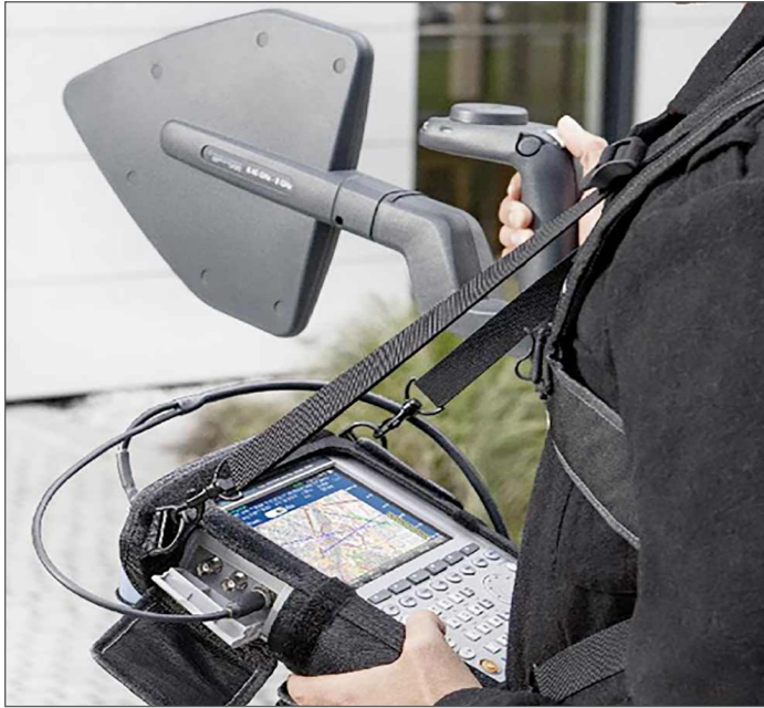
Figure 7: The Rohde & Schwarz R&S®PR100 custom spectrum analyzer with mapping and triangulation and R&S®HE300 antenna. The R&S® FSH analyzer may also be used. Photo courtesy, Rohde & Schwarz.
