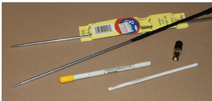
Figure 3. Metal and plastic knitting needles may be used to test for RF energy on connector pins. Plastic crochet hooks can manipulate cables without having to touch them.
