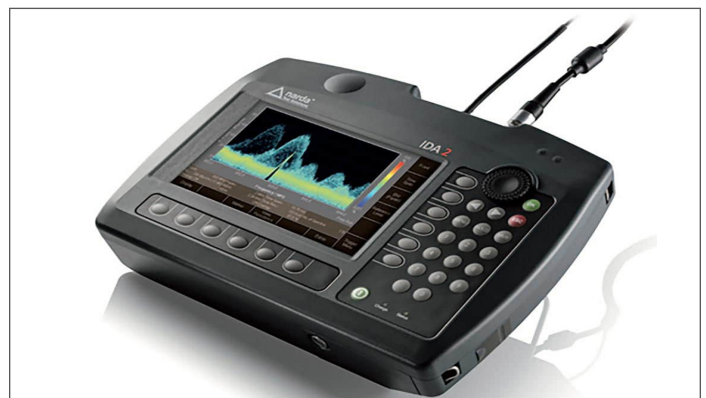
Figure 5: The Narda IDA2 spectrum analyzer and interference hunting system. The frequency range is 9 kHz to 6 GHz. Photo, courtesy Narda STS.
