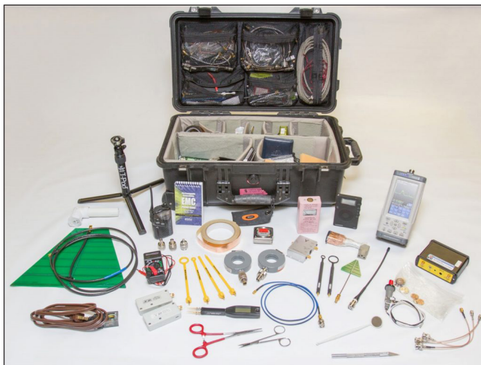
Figure 1 - Troubleshooting kit with most of the major components shown. The spectrum analyzer is the Thurlby Thandar model PSA6005 and tunes from 10 MHz to 6 GHz. Everything fits inside a Pelican 1514 roller transit case. The contents are described in Part 1 and Part 2 of this article
