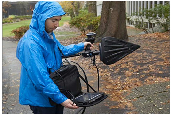
Figure 9: The Tektronix spectrum analyzer with mapping/triangulation and Alaris DR-A0047 antenna. Photo, courtesy Tektronix.
