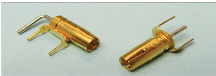
Figure 12 - An example of miniature oscilloscope probe sockets for high-frequency measurements. These eliminate the issue of long ground leads that can compromise the signal measurement and cause ringing. They are typically soldered directly to the PC board under test. The spring-loaded oscilloscope probe tip is pulled off and the tip is inserted directly into the socket.
