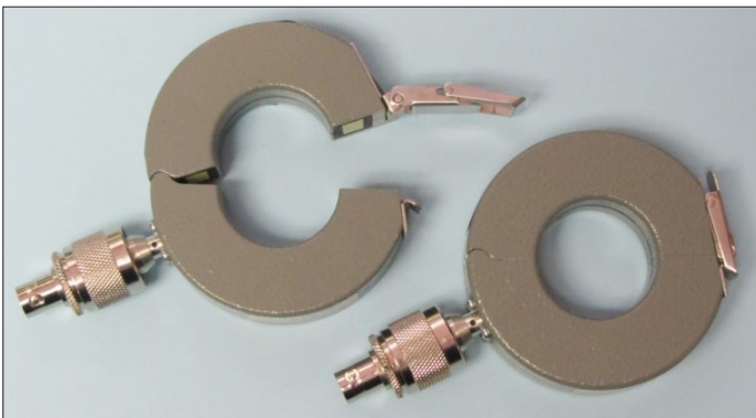
Figure 14 – A matched set of clamp-on Fischer Custom Communications model F-33-1 current probes. While not imperative to purchase, a matched set is very useful for advanced troubleshooting I/O cable emissions. They can sense RF currents of a few microamps.
