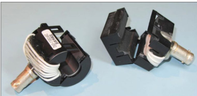
Figure 13 – An example of simple current probes you can make to measure harmonic RF currents in cables.
