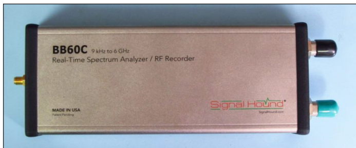
Figure 8 - The Signal Hound BB60C USB-controlled real-time spectrum analyzer covers 9 kHz to 6 GHz and has a real-time bandwidth of 27 MHz. The cost is $2,879.
