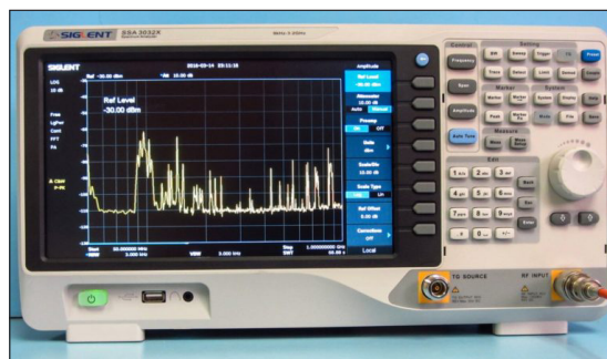
Figure 5 - The new Siglent SSA3000X-series spectrum analyzer tunes from 9 kHz to 2.1 GHz or 3.2 GHz, depending on the model.
