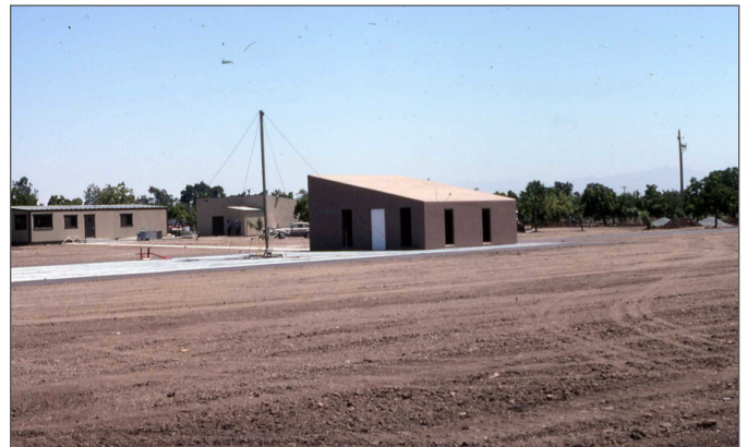
Figure 2 - A typical open area test site (OATS).
