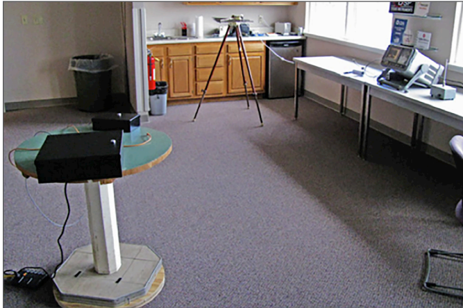
Figure 2. An example of a 3 m pre-compliance test set up in a large conference room. Note the DIY turntable for helping maximize emissions.
