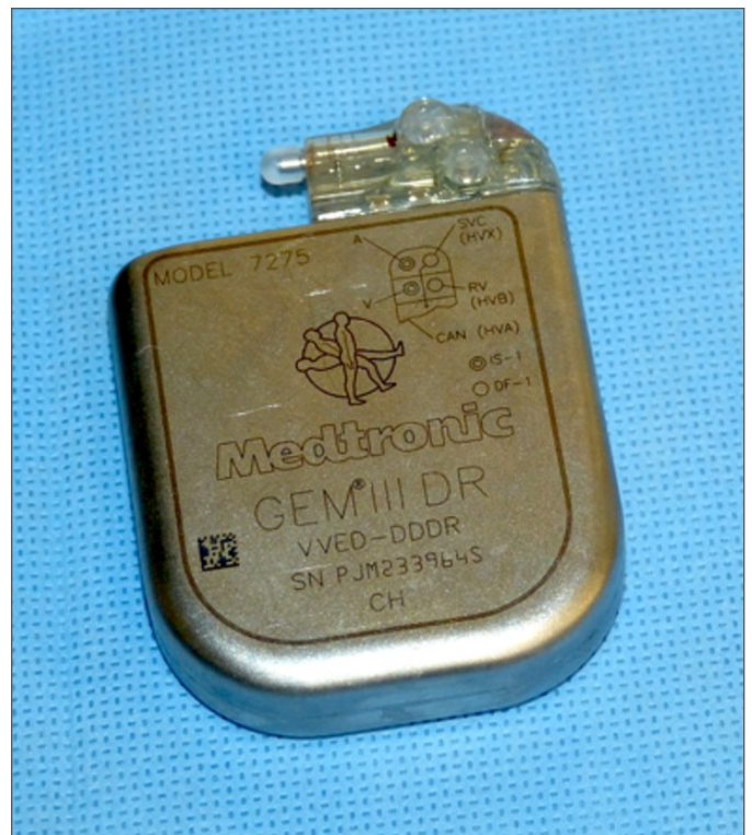
Figure 8: Implantable medical devices like the pacemaker shown here have understandably exacting mechanical and electrical performance requirements for every component specified as part of the system.
