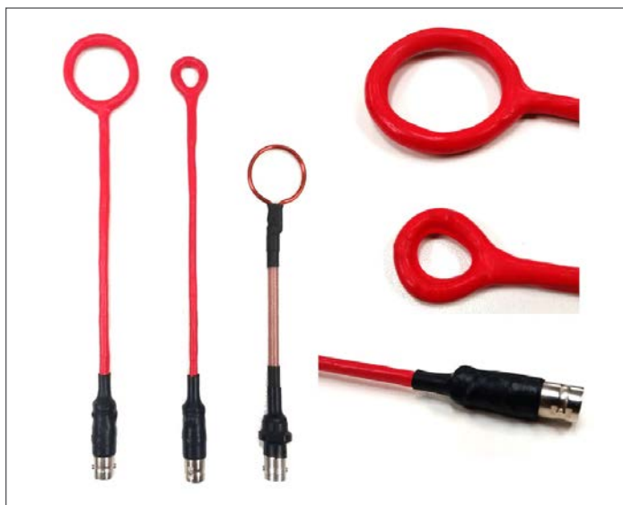
Figure 1: H-field probes. At right details of the ones that I made myself.
