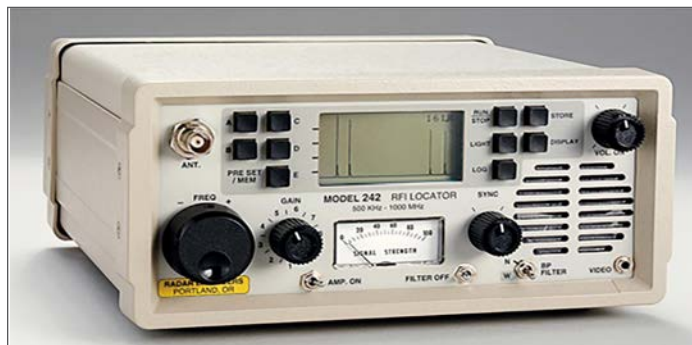
Figure 2: A signature analyzer from Radar Engineers that tunes from 500 kHz to 1 GHz and which displays an electronic “signature” of a specific interference source. Receivers such as this are used by professional investigators to track down power line noise. (Image Source: Radar Engineers).
