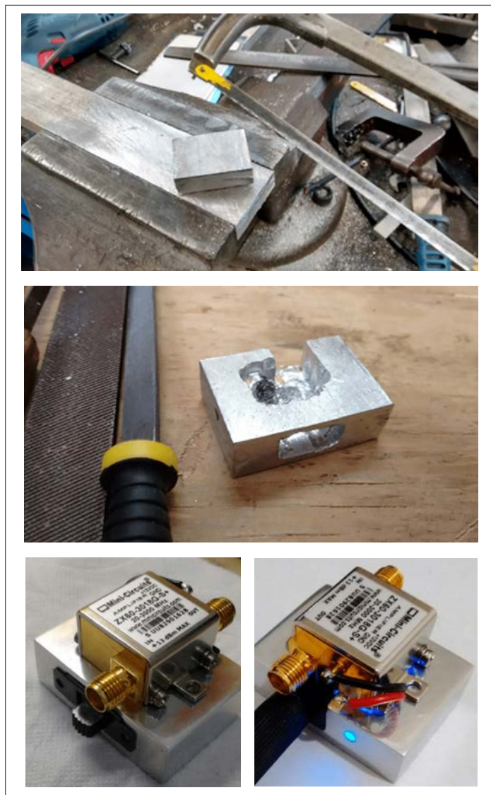
Figure 7: Making the amplifier: from the aluminum chunk to the shiny assembly
