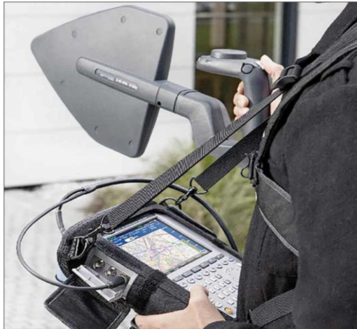
Figure 7: The Rohde & Schwarz R&S®PR100 custom spectrum analyzer with mapping and triangulation and R&S®HE300 antenna. The R&S® FSH analyzer may also be used. Image Source: Rohde & Schwarz.
