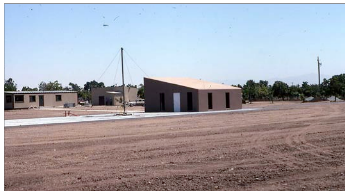
Figure 2: A typical open area test site (OATS).
