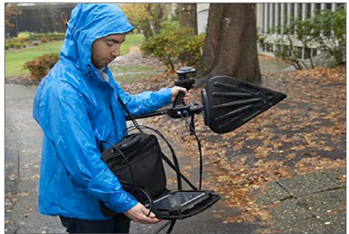
Figure 9: The Tektronix spectrum analyzer with mapping/triangulation and Alaris DR-A0047 antenna. Image Source: Tektronix.
