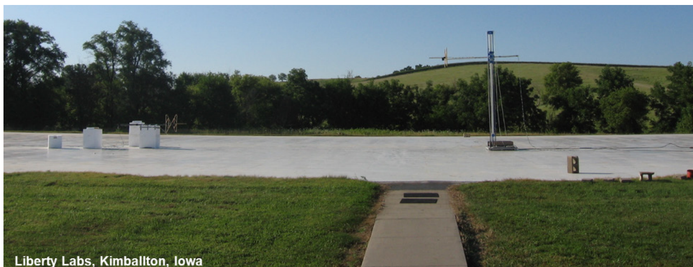
Image 1 - Liberty Labs in Kimballton, Iowa; An example of an EMC open area test site
