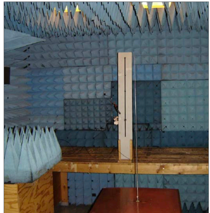
Figure 4—A monopole and small isotropic bow tie antenna in a well-damped chamber.
