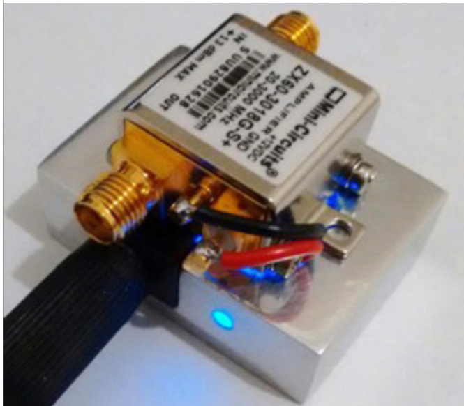
Figure 7 - Making the amplifier: from the aluminum chunk to the shiny assembly
