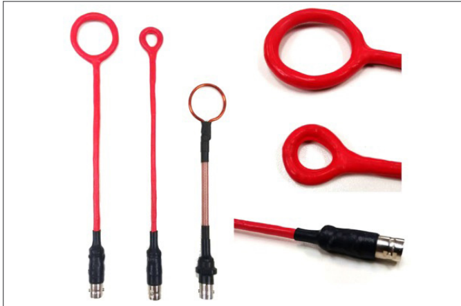
Figure 1 - H-field probes. At right details of the ones that I made myself.
