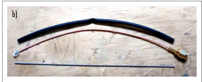
Figure 5 - a) Inner conductor soldered to braid forming a loop; b) Shrinkable sleeve, probe and twisted rod
