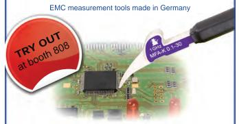
The MFA- micro probes (near-field probes) have a very small probe head that functions like a coupling clamp. It allows the current measurement at finest conducting paths and IC pins.
