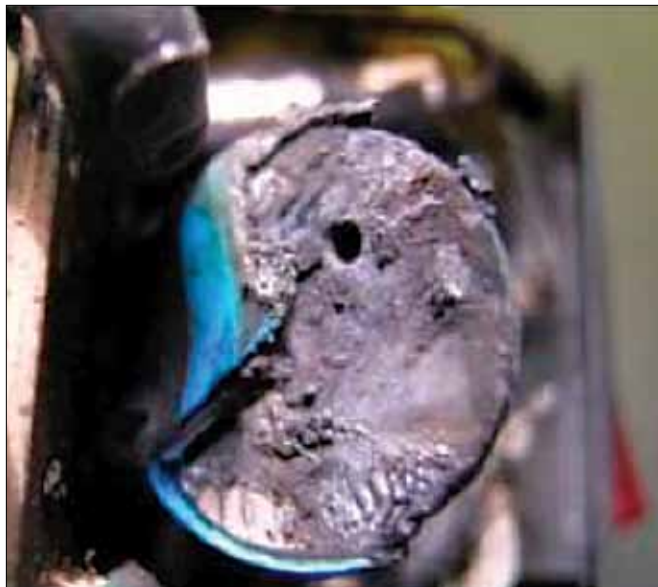
Figures 3 and 4. (Left and right) MOV after a thermal runaway condition occurred inside a consumer electronic device.
