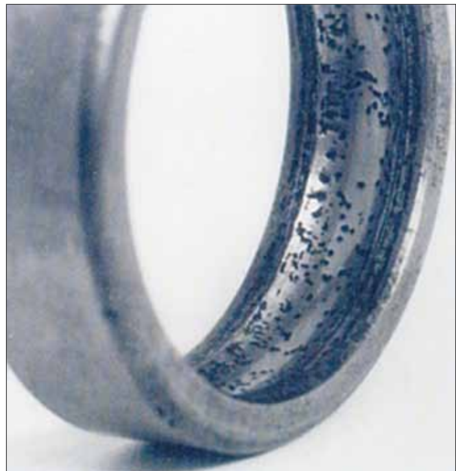
Figure 5. Example of bearing corrosion as a result of transient arcing.
