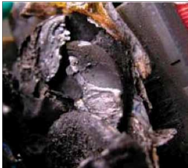
Figures 3 and 4. (Left and right) MOV after a thermal runaway condition occurred inside a consumer electronic device.
