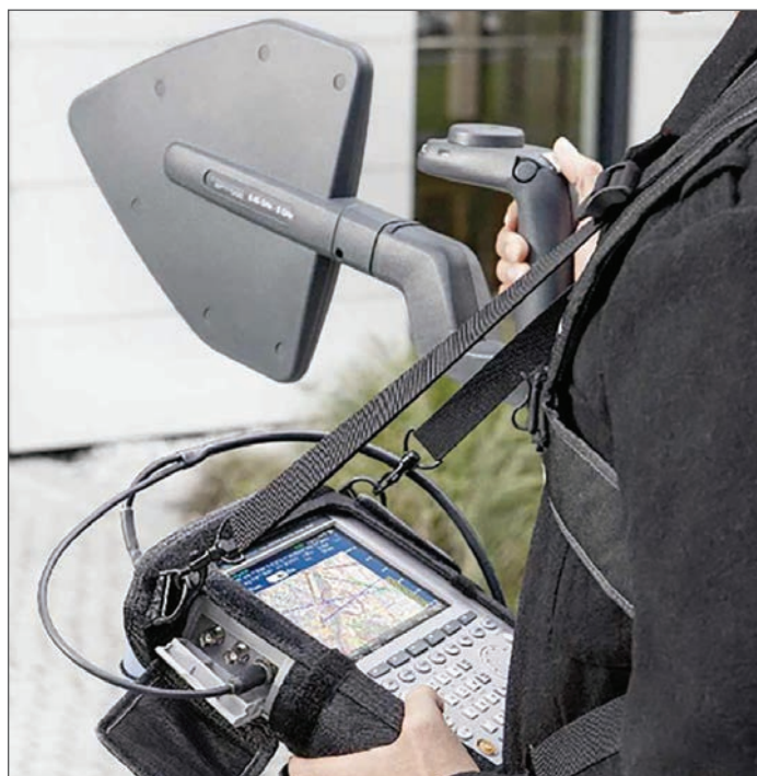
Figure 7. The Rohde & Schwarz R&S®PR100 custom spectrum analyzer with mapping and triangulation and R&S®HE300 antenna. The R&S® FSH analyzer may also be used. Photo courtesy, Rohde & Schwarz.
