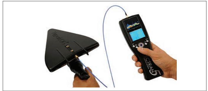
Figure 3. The Aaronia Spectran V5 handheld real-time analyzer is the smallest self-contained unit and tunes from 9 kHz to 6 GHz. Other models have upper frequencies of 12 and 18 GHz.
