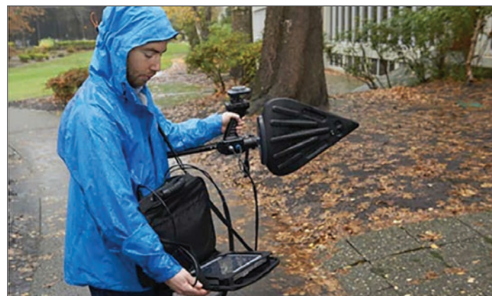
Figure 9. The Tektronix spectrum analyzer with mapping/triangulation and Alaris DR-A0047 antenna. Photo courtesy, Tektronix.
