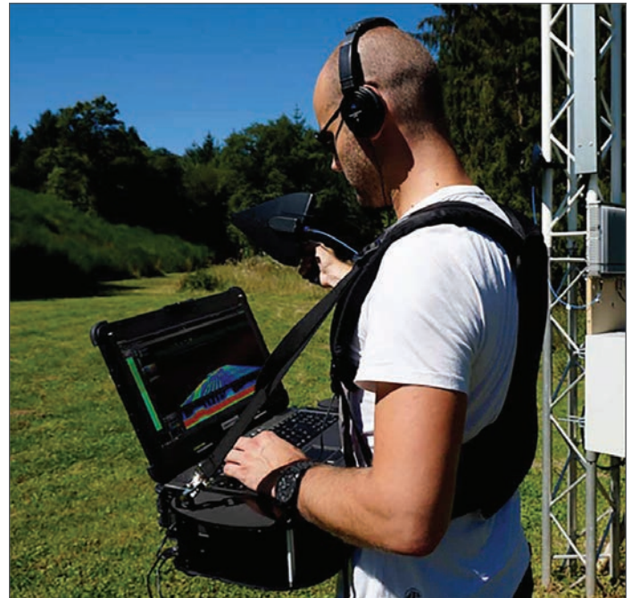
Figure 4. The Aaronia Spectran V5 XFR PRO in the field portable configuration.
