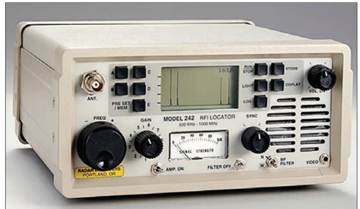
Figure 2. A signature analyzer from Radar Engineers that tunes from 500 kHz to 1 GHz and which displays an electronic “signature” of a specific interference source. Receivers such as this are used by professional investigators to track down power line noise (photo courtesy, Radar Engineers).
