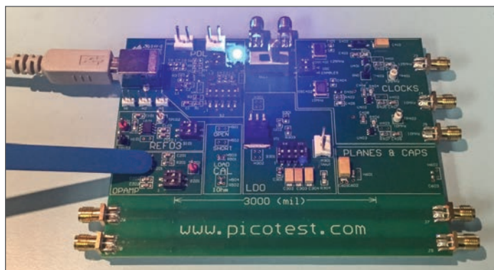
Figure 7 – Measuring an op-amp on the Picotest Technologies demo board.
