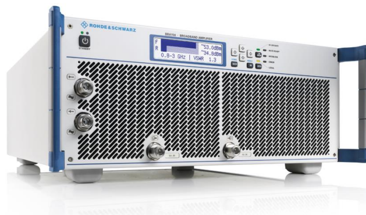
Figure 2 - Broadband amplifier used in immunity testing
