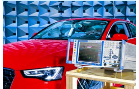
CISPR 25 covers interference caused by the vehicle to equipment mounted within the vehicle, such as a radio or GPS receiver.
