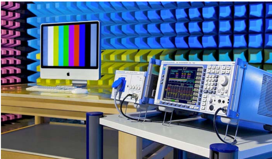
Conducted EMI test in accordance with CISPR 32 for a television receiver.
