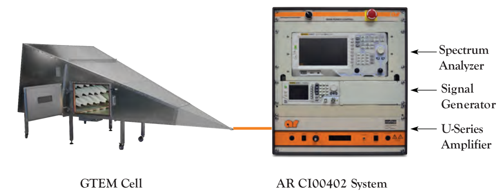
AR GTEM Cell RI Test Setup
