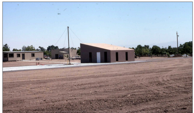
Figure 2 - A typical open area test site (OATS).
