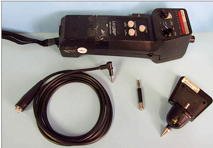
Figure 9. A typical ESD simulator with air and contact discharge tips. It can produce up to +/- 15 kV.
