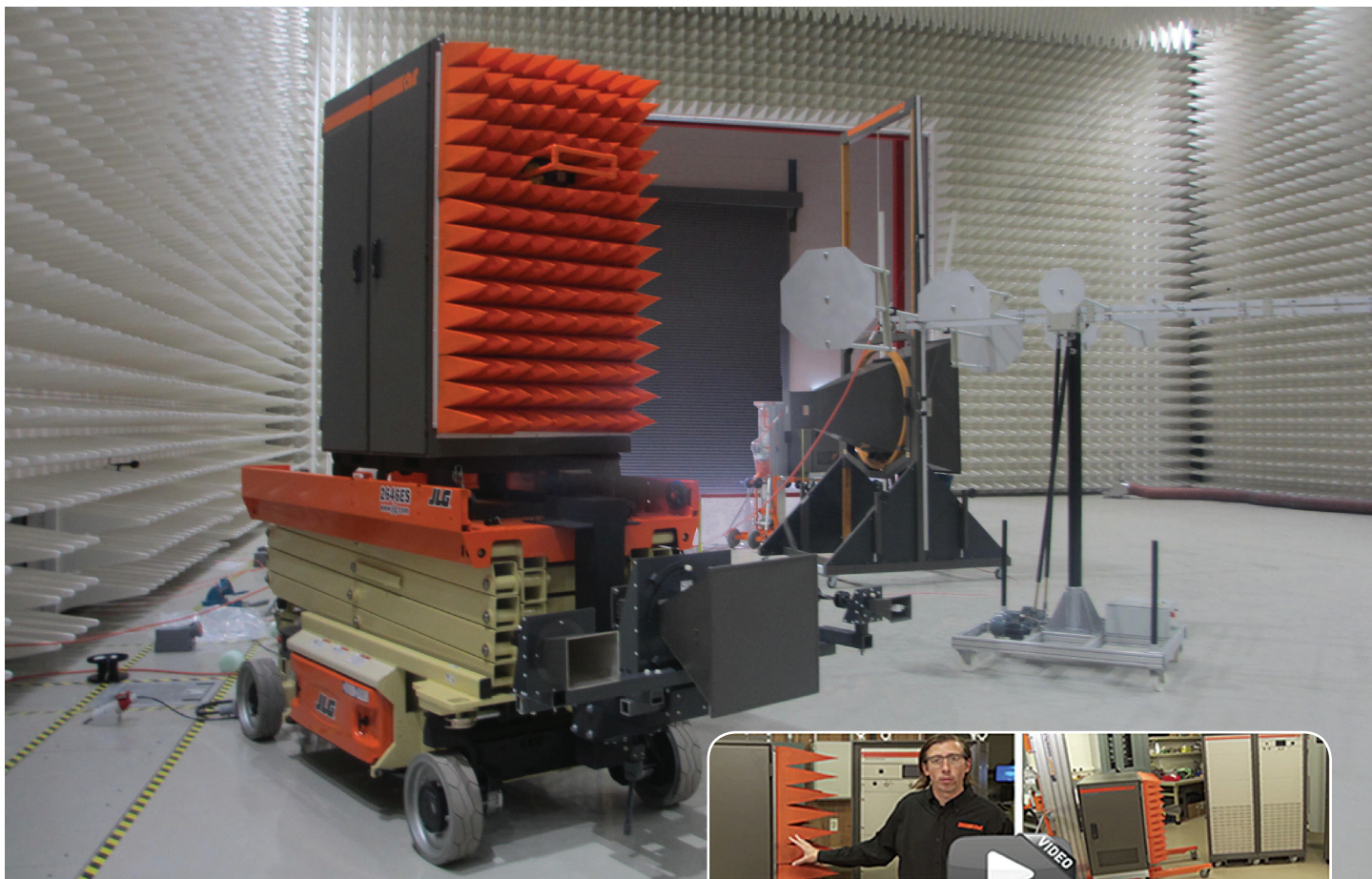
SP1053 1-18 GHz, 200V/m, Radiated Immunity System on an electric scissor lift with a 1-6m adjustable antenna height.
