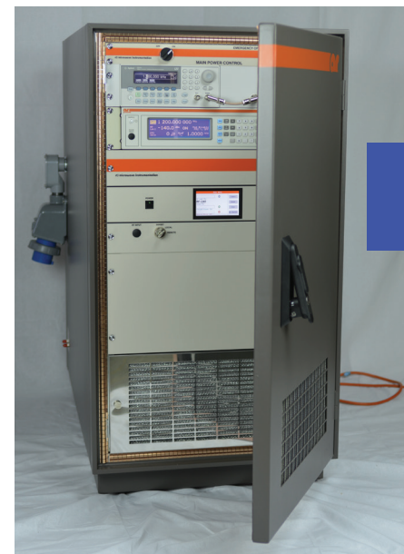
Shielded radiated system allows operation inside chamber during radiated immunity testing.
