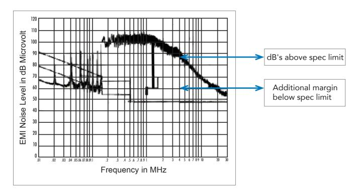
Minimum Total Insertion Loss = (dB's above spec limit) + (Additional margin below spec limit)
