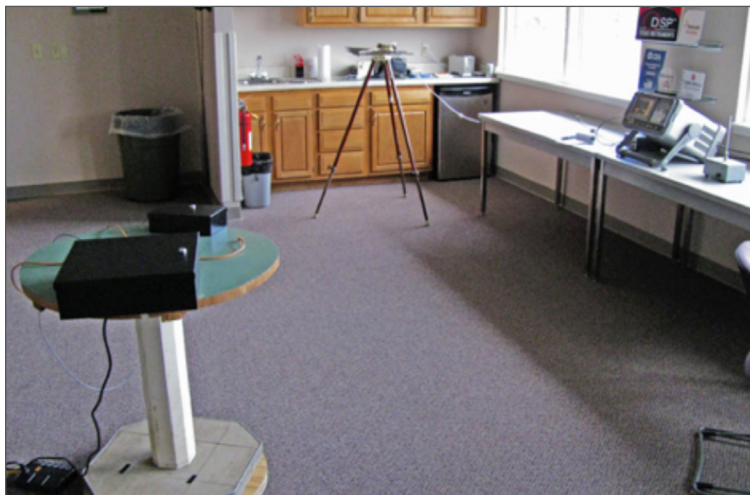
Figure 3 - An example of a 3m pre-compliance test set up in a large conference room. Note the DIY turntable for helping maximize emissions.
