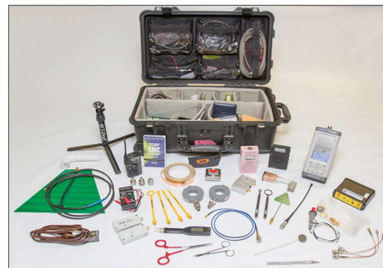
Figure 1 - The troubleshooting kit I've developed over the years can characterize and debug many emissions and susceptibility issues.
