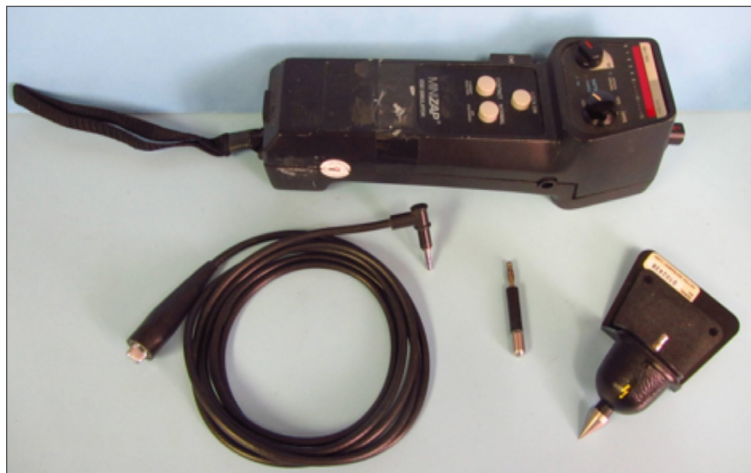
Figure 8 - A typical ESD simulator with air and contact discharge tips. It can produce up to +/- 15 kV.
