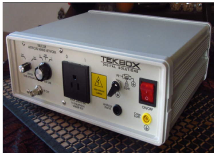
Figure 1 - A typical line impedance stabilization network, or LISN.
