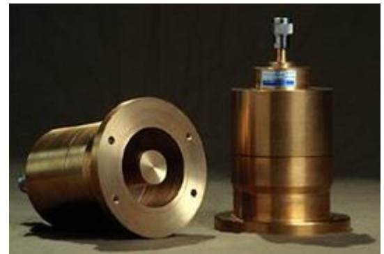
Fig 1. ASTM D4935-10 test fixture for SE measurements at f= 30 MHz - 1.5 GHz.
