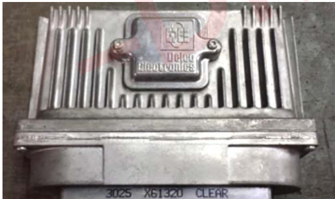
An Engine Controller Unit (ECU) from a 1996 Chevrolet Beretta courtesy of Delco Electronics and Wikipedia.
