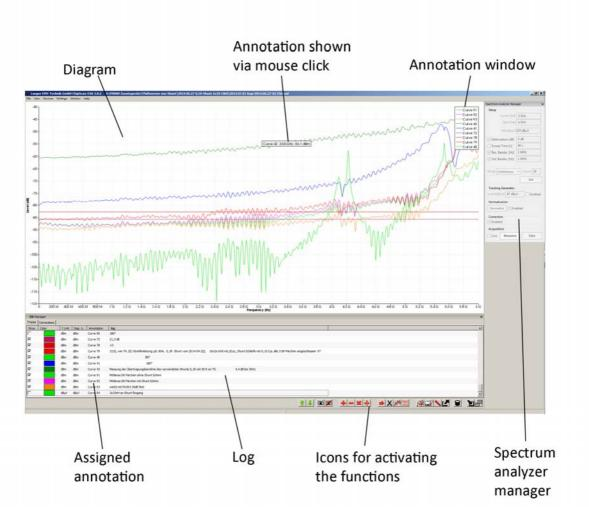
The ChipScan-ESA software has been developed primarily for measurements in the field of electromagnetic compatibility (EMC). It
