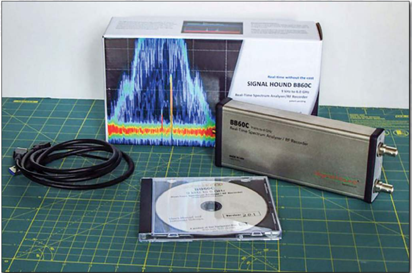
Figure 15 – The Signal Hound BB60C USB-controlled real-time spectrum analyzer, shown with supplied accessory. The unit is small enough to be Velcro'd to the lid of a laptop.
