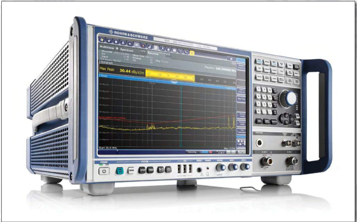
Figure 13 – Rohde & Schwarz offers their new ESW EMI test receiver with 80 MHz real-time capture (shown in the figure) with touchscreen control, and includes models that cover 2 Hz to 8/26/44 GHz. All models include a very fast FFT-based time domain scan, which can be run with two CISPR detectors to record parallel measurements. In addition, the new ESW includes special notch filters for the 2.4 and 5.6 GHz ISM bands, to help prevent signal overload when making sensitive measurements outside, but near, these bands. Other models include the FSVR and ESR3/7/26 that can range in frequency from 9 kHz (10 Hz option on FSVR) to 3.6/7/26.5 GHz. Real-time bandwidths are 40 MHz for all models. Base prices range from $50,000 to $77,000. Image courtesy Rohde & Schwarz.
