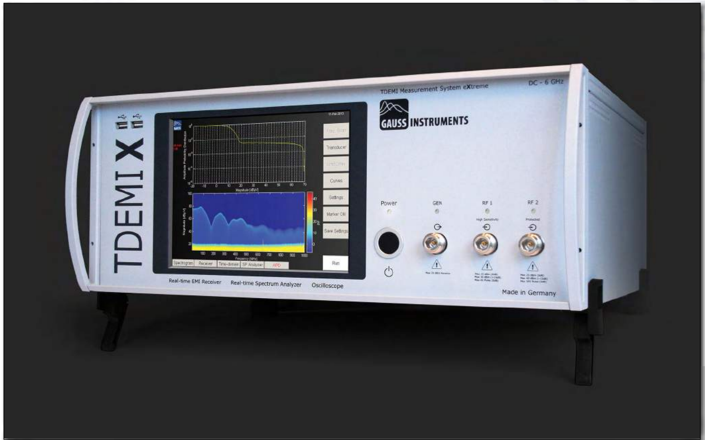
Figure 11 – Gauss Instruments was one of the pioneers of the real-time FFT analyzer. They currently have three model series that start at 10 Hz and go up to 1/3/6/26.5/40 GHz (depending on model). The real-time bandwidths are 162.5 MHz and 325 (645 MHz option) for the “X” series. Base prices range from $25,000 to $50,000. Image courtesy Gauss Instruments GmbH.
