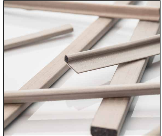
Figure 5: Metalized fabric gaskets from Orbel are manufactured with a polyurethane foam core and nickel-plated copper-conductive fabric.
