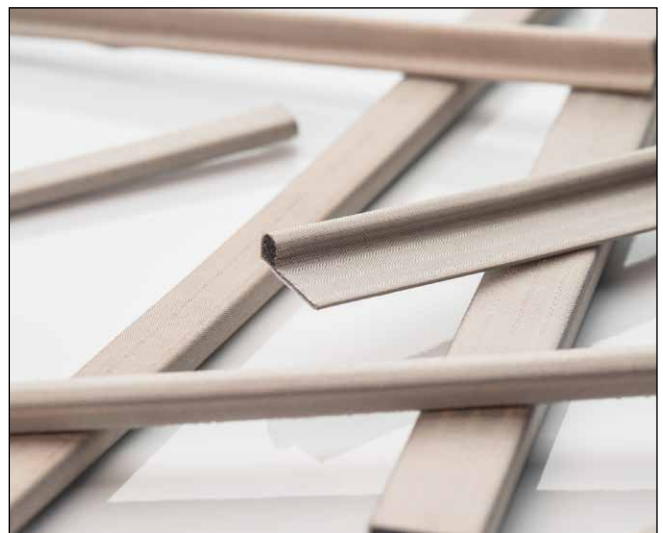
Figure 4: Metalized fabric gaskets from Orbel are manufactured with a polyurethane foam core and nickel-plated copper-conductive fabric.
