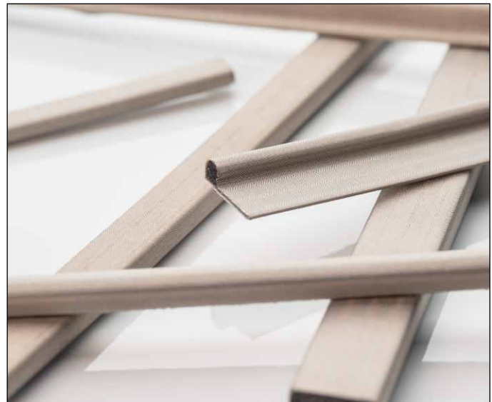
Figure 4: Metalized fabric gaskets from Orbel are manufactured from a polyurethane foam core and wrapped with nickel-plated copper-conductive fabric.
