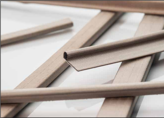
Figure 3: Ideal for the control of EMI, conductive fabric gaskets from Orbel are manufactured from a polyurethane foam core and wrapped with nickel-plated copper-conductive fabric.
