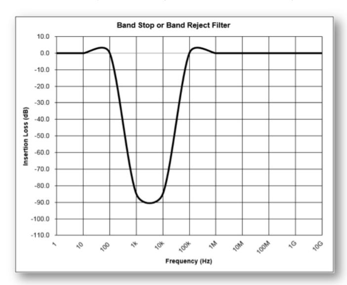
pass through the circuit, but provide high impedance to the frequency signals within a certain range. This attenuates (lowers the magnitude of) the signals within this specific frequency range as shown in the example graph below.
