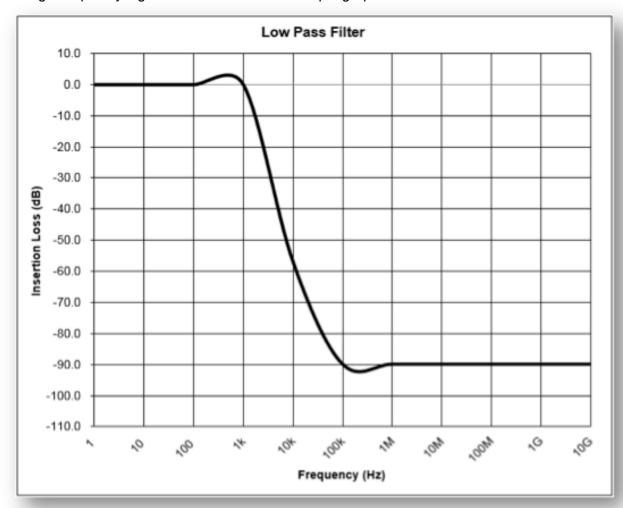
Generally AC Power systems run at either 50 Hz, 60 Hz or 400 Hz, so all Genisco Power Filters are Low Pass Filters. Our filters allow the lower frequency power signals to pass through the circuit, and block the unwanted higher frequency noise.
