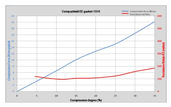
\*Test is made on Compashield EE gasket model 1516. Tests result for other profiles or dimensions are available based on request. Recommended compression degree 10% to 30% in the assembled state.
