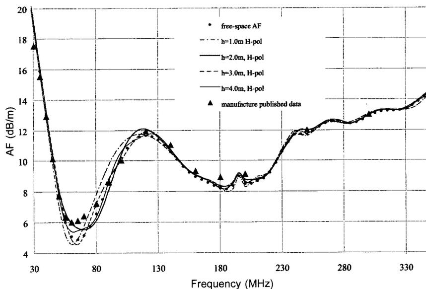
**Figure 2. Horizontal AFs of a traditional bicon/log hybrid antenna at different heights above a conducting ground plane.**
