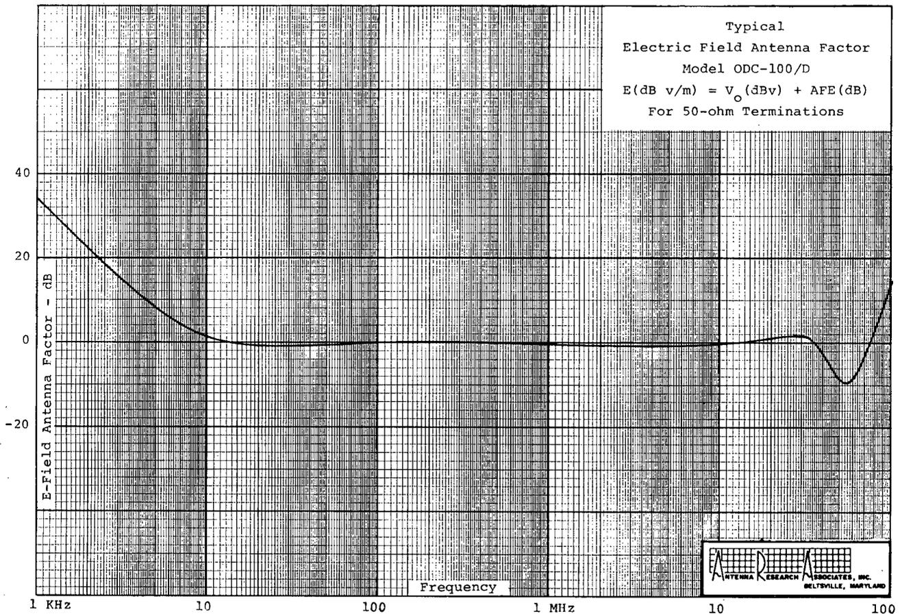
One of the whip antennas offered by Antenna Research Associates is the ODC-100/D, whose physical height is about 62 inches, and whose effective whip height is about 0.79 meters. Its preamplifier has a gain of approximately 10 dB. Substituting in (8) for  $h_e$ , one obtains a response of
