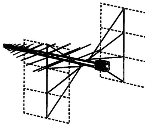
**Figure 1. A bicon/log hybrid antenna for both emissions and immunity measurement—(dashed parts removed for radiated emissions measurement, or dashed parts installed for radiated immunity test).**
