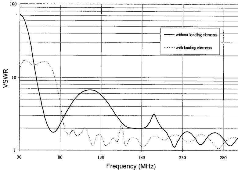
**Figure 4. Numerically modeled voltage standing wave ratio of a traditional bicon/log hybrid antenna and a bicon/log hybrid antenna with capacitive loading elements**
