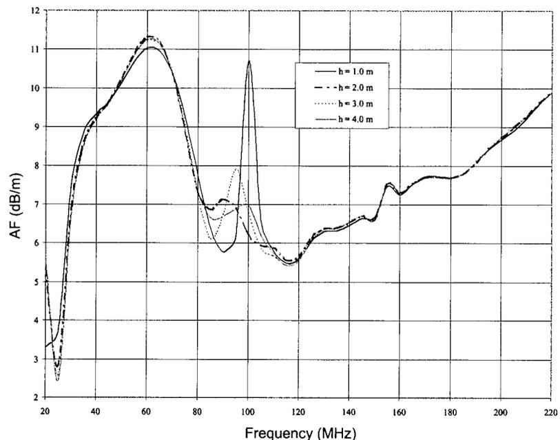
**Figure 5. Numerically modeled AF for a vertically polarized bicon/log hybrid with L-shaped capacitive-loading.**
