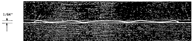
At least nine lines of contact occur when the gasket is compressed to 1/64". (Note: Recovery from this deflection is excellent. See top illustration.)
