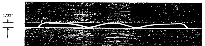
At 1/32" gap the tips of the fingers are in contact with the mounting surface, and the center arch is in contact with the closing surface, making a total of seven lines of contact.
