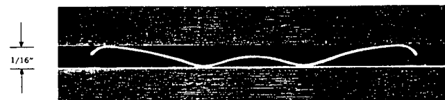
Note increased arching of center at 1/16" gap. This produces wiping contact with the mounting surface.
