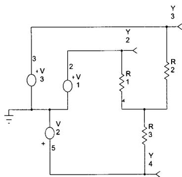
**Figure 1. Schematic representation of a 120/208-volt 3-phase wye system configured with a "lifted neutral" connection.**
