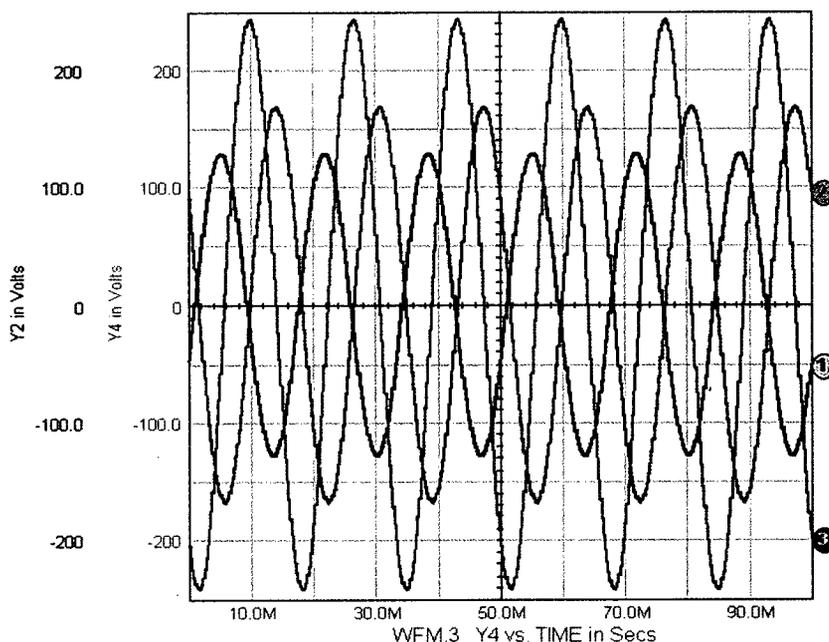
**Figure 2. Computer simulation of the phase-to-neutral voltages of a 120/208-volt, 3-phase wye system configured for a "lifted neutral" event. Phase A (1) current at 100 amperes (100%), phase B (2) current at 75 amperes (75%), and phase C (3) current at 10 amperes (10%).**
