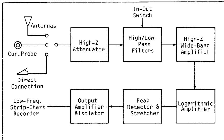
Figure 1 Block Diagram of Typical Transient Detector and Recorder
