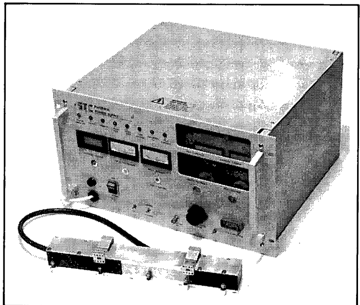
Figure 2. MM Wave TWT and Power Supply.
