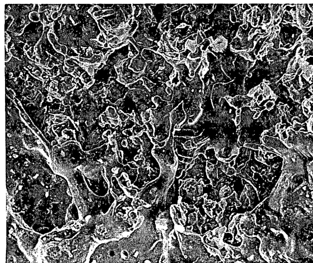
Figure 3. A sprayed-on metal coating. Scale 1000 to 1
