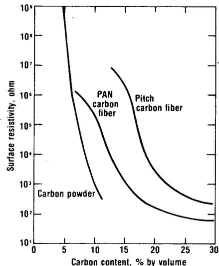
*Carbon-powder composites are more conductive than carbon-fiber composites. But resistivity of carbon-fiber composites varies less as carbon volume fluctuates.*
