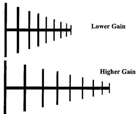
**Figure 4.** Log Periodic Antennas with Equal Bandwidth.
