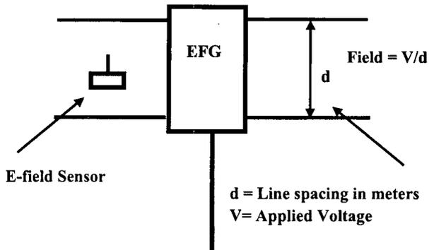
Figure 7. E-field Generator (EFG).
