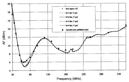
Figure 3. Vertical AFs of a traditional bicon/log hybrid antenna at different height above a conducting ground plane.
