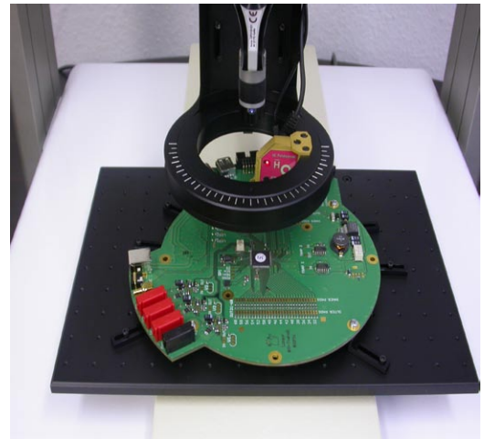
A circular solid state circuit board is mounted on the PCB holder and fixed with claw fasteners.
