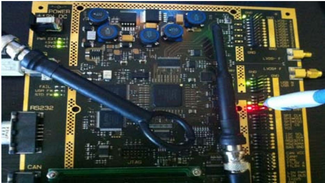
Figure 2 Rohde & Schwarz offers a family of near-field E and H field probes (or “sniffer” probes R&S®HZ15) which can be used to diagnose the cause of an electromagnetic interference problem.
