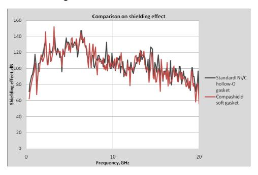
\*Test is made on gaskets in dimension 4,0mm x1,5mm as reference. Compashield Soft gasket has the same excellent shilding properties as the standard Ni/C hollow-o gasket.
