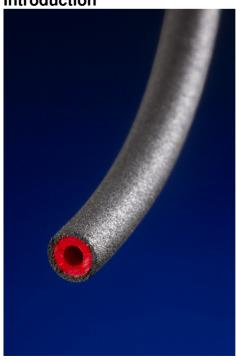
Compashield Soft is an EMI shielding gasket developed by Nolato. It's a modified version of standard one material hollow-O gasket. It is co-extruded with conductive material as the outer layer and non-conductive material as the inner layer.
