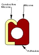
For easier handling in case of transportation Compashield EE gasket can be mounted onto the flange by using a double-coated adhesive tape on the back side. Remove the release film and position the gasket using light pressure. When the gasket is properly positioned, firmly press onto the flange.
