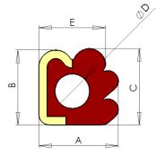
Compashield EE gasket with 'hook' is an improved version of the standard EE gasket. This solution offers several benefits. The gasket could be fixed in place without back tape and offers an extremely good shielding effect thanks to the unique design.
